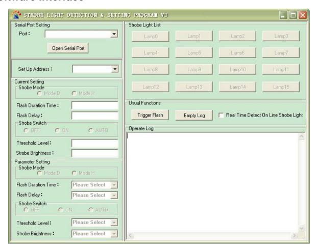
1. **Port:** Click the drop-down list choose control PC and Serial port of LED Strobe light, make sure communication is normal controlling.
