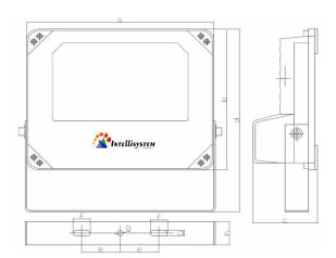
a: 261mm b: 261mm c: 90mm d: 322mm e: 54mm f: 24mm
